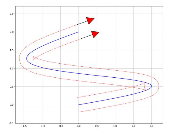
The generated paths can get a bit more interesting when trying to make tight turns. The path shown above sends negative velocities to the inner wheel during the turns in order to make turns in a small space.
