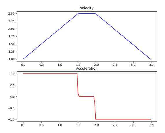
The robot's *Constraints* provide the maximum allowable dynamics for the generated paths. Careful measurement and configuration of these parameters ensures that the path will not expect the robot to move more quickly than it actually can. Resolving such discrepancies in the generated path and reality is an important first step in ensuring that the robot performs reliably.
